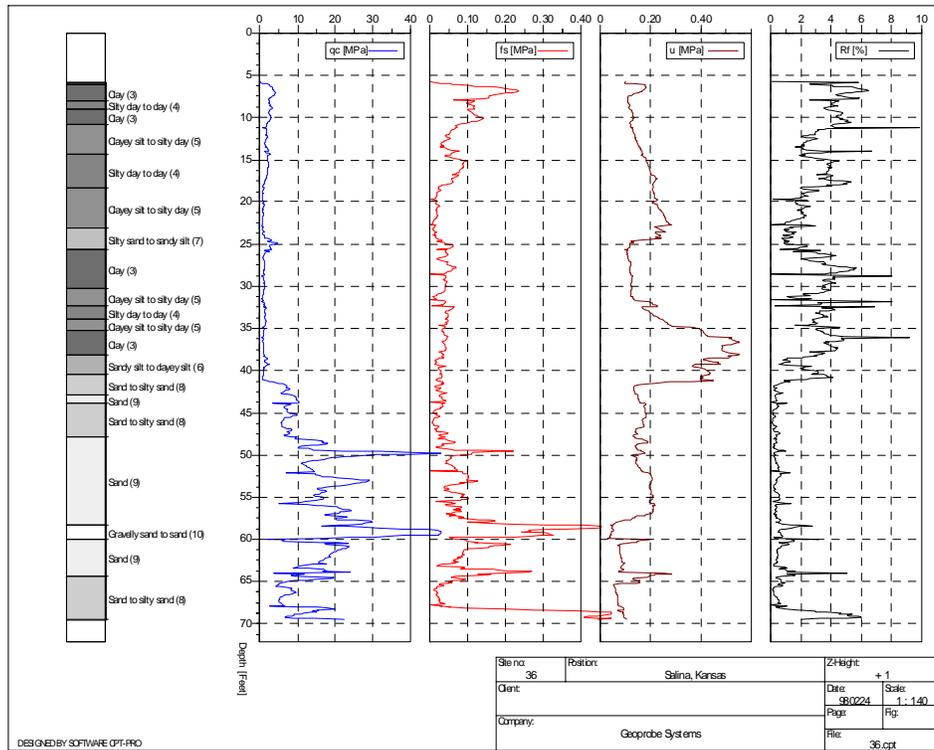
Figure 4. A CPT log from Salina Kansas. Equipment: Geoprobe soil probing unit pushing a Geotech AB cordless CPT probe.  $q_c$  = tip resistance,  $f_s$  = sleeve friction,  $u$  = pore pressure, and  $R_f$  = friction ratio.
