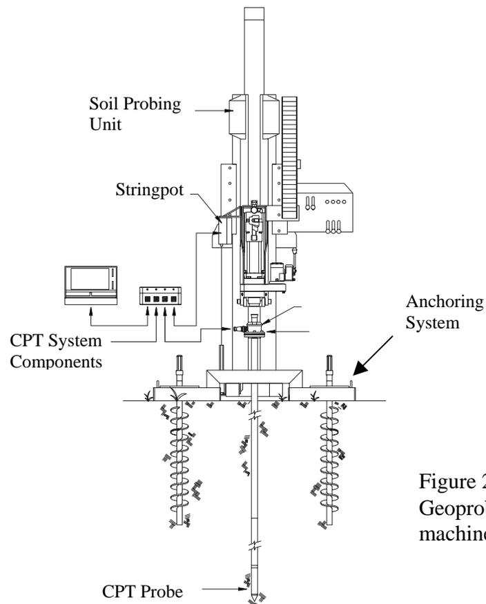
Figure 2. Anchored Geoprobe<sup>®</sup> soil probing machine with CPT.
