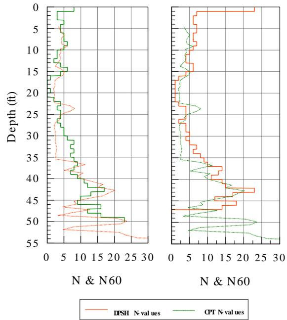
Figure 11. DPSH results compared to SPT N-values that were calculated using CPT N<sub>60</sub> results.
